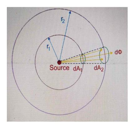
As per the above figure, the two radiuses are  $r_1$  and  $r_2$ . At distance  $r_1$  dA<sub>1</sub> is the elementary surface area taken. In this direction of dA<sub>1</sub>, dA<sub>2</sub> is considered at  $r_2$  distance.
