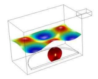
Potato in a microwave: Electric field and temperature plot. The rectangular block on the right represents a waveguide feed.
