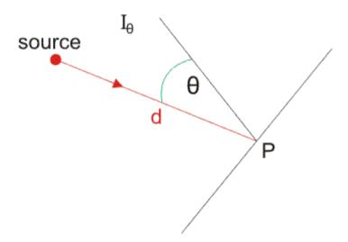
But for non point source, the cosine law of Illuminance can be analyzed in term of luminous flux instead of luminous intensity.
